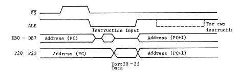
Fig. 8(b) Single Step Operation Timing
