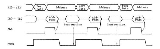
Fig. 5 Timing of External Program Memory Access
