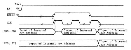
Fig. 7 Timing of Rading Internal Program Memory
