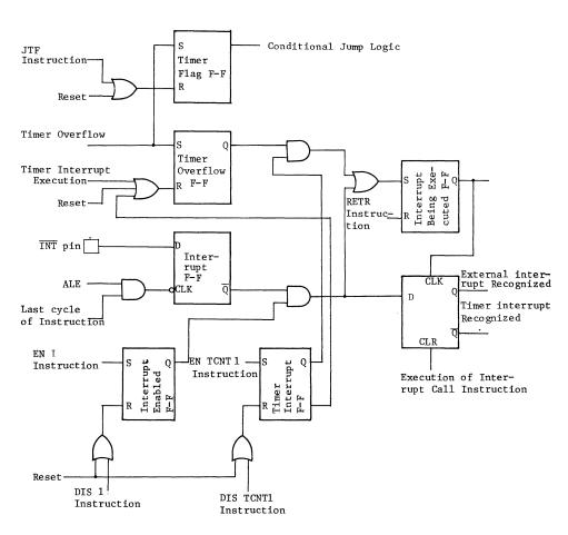
Fig. 3 Concept of Interrupt Control Circuit
