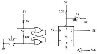
Fig.8(a) Single Step Circuit
