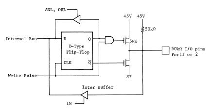
Fig.1 Input/Output Circuit of Port 1, Port 2
